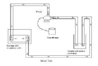
Light source : Quark's Excimer Lamp 222nm Dia.18mm x L290mm One Lamp power : 50W x 1
