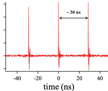
**Figure 3** Reduced repetition rate with an extra length cavity. The repetition rate changed from 98 MHz to 35 MHz.
