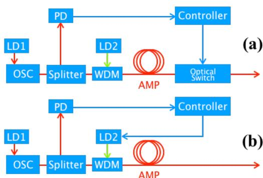
**Figure 1** Schematic of pulse picking laser system. (a) ordinal pulse picking system with optical switch and (b) direct modulating pumping LD system.
