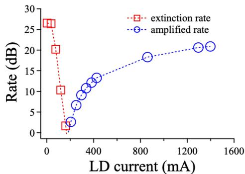
**Figure 2** Extinction and amplified rate with 1030 nm laser at 98 MHz. The extinction rate of 25 dB was achieved.
